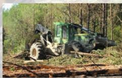
**Cut-To-Length Operation** – An operator within a cab with computerized measurement capabilities severs the standing tree and, still gripping it with a processor-head, strips off the limbs, and cuts it to specified lengths. A wheeled or tracked forwarder then picks up the processed pieces and transports the load to the landing. A loader then transfers the fully processed logs to the truck for transport.
